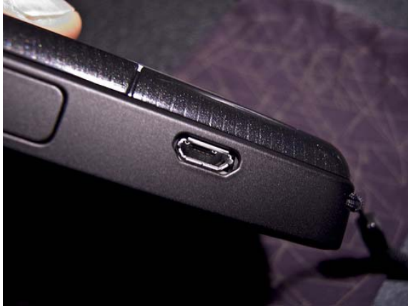
Figure 4: Micro USB receptacle in a mobile phone
